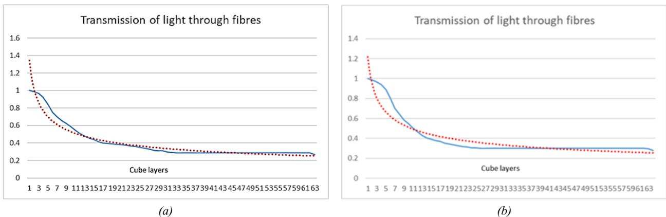
**Figure 4.** The ray tracing simulation of light propagation in the modelled sample of washi-like paper. (a) Graph of the normalized light intensity (in blue) and power fit of the data (red dots). (b) graph of the normalized intensity of linearly polarized light (in blue) and power fit of the data (red dots)
