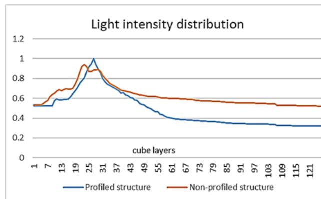
**Figure 5.** The ray tracing simulation: graphs of the resulting data in the layers of the cube. The light intensities normalised according to values of the profile model are shown on the vertical axis. The area between the layers 4 and 28 represents the region of the model inside the cube
