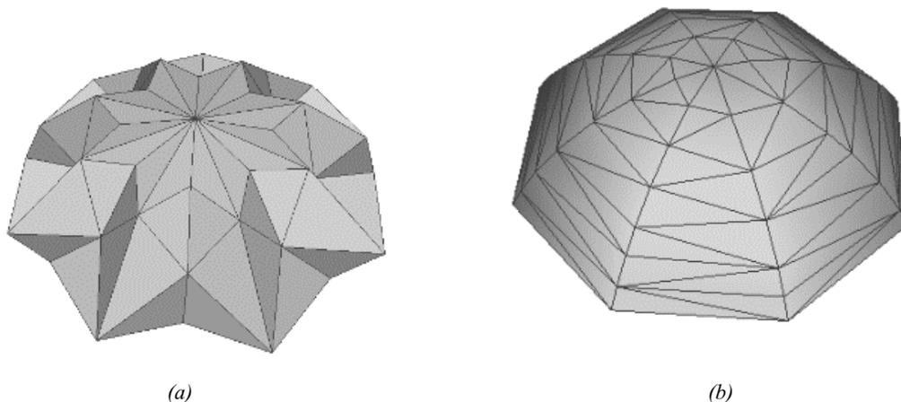
**Figure 1.** Geometry models [1]. (a) The profiled polygonal model. (b) The non-profiled polygonal model
